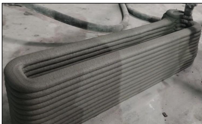
Figure 9. 3D printed object using CM-12 mix
