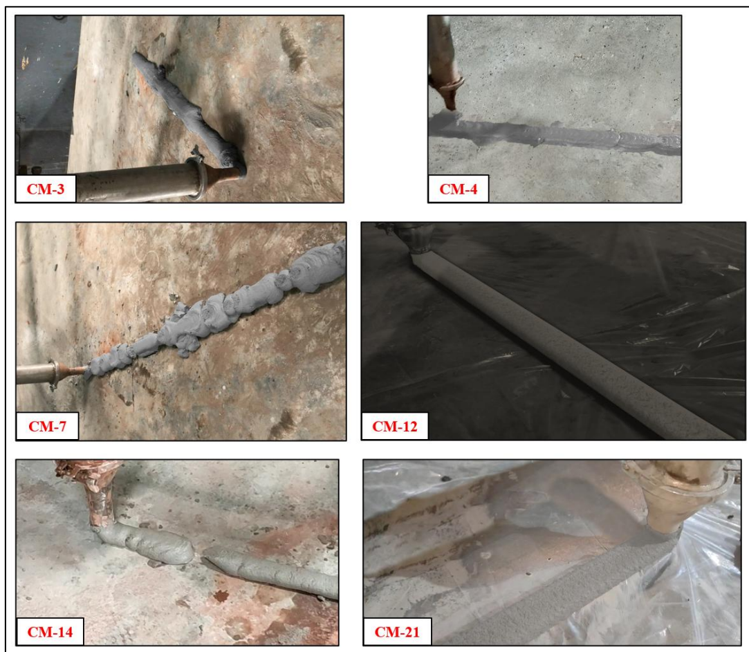
Figure 8. Visual examination for printability evaluation of the printable zone mixtures.
