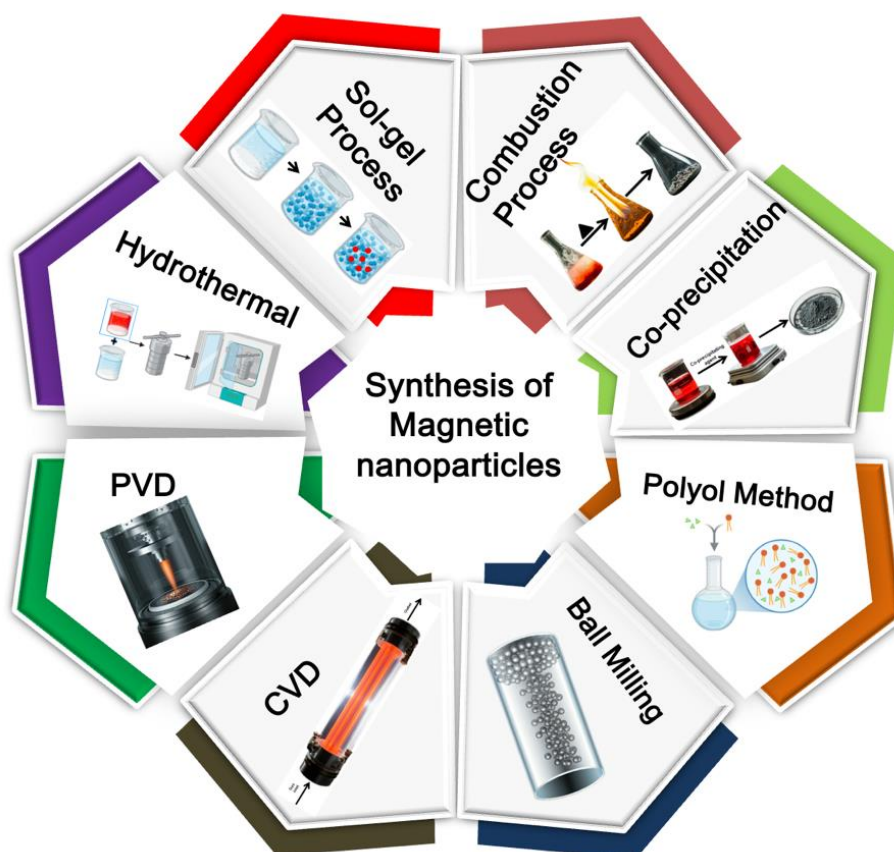
Figure 3. The various synthesis methods of magnetic nanomaterials
